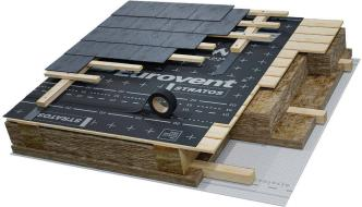
slot between the membrane and the thermal insulation (mineral wool, fiberglass) is not required for installation – the product can be installed directly on thermal insulation. The final roof covering must be assembled with batten and counter-batten. Suitable for use in nearly all types of roof coverings – recommended for ceramic, concrete, metal roofing tiles, aluminium sheets, etc.
